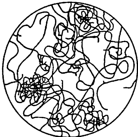
Fig. 18. Schematic presentation of the macromolecular (or matrix) structure of a lightly cross-linked polymer bead.
